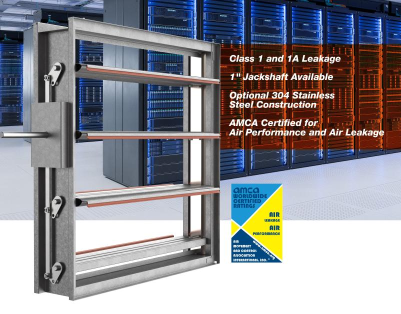
Pottorff's **CD-45** (parallel blade) and **CD-46** (opposed blade) control dampers feature high-performing airfoil blades and a rugged hat channel frame to provide exceptional air control in medium to high pressure and velocity applications. They are a great solution for regulating airflow and reducing energy consumption for Data Centers, Warehouses and Distribution Centers.
